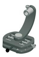
Using the swivel and tilt adapter you can align the laser level, irrespective of the surface below. The Adapter also allows for a parallel movement which is very useful when aligning the laser parallel to a reference object. The Adapter is accomodated with a 5/8" thread, and is also fitted with a three-point magnet arrangement underneath.
