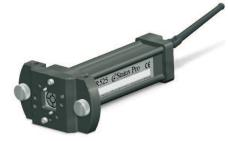
The R525 is a rugged but precise 2D Laser-Position detector. It was developed originally for machine tool alignment applications. Because of the Wireless interface and its versatility it used today in a multitude of applications. Together with the ProLineV2 Software application we measure XY and Z simultaneously. If we use the T330 as a laser source we have a reference which automatically levels itself. These features together are very powerful and save a great deal of time on-site.
