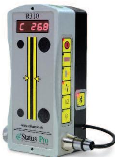
The R310 measures the position of the rotating laser beam. The CCD Sensor has total measurement range of 80mm. The beam forms an entire reference plane. The R310 is wireless and can measure up to a distance of 80m from the Laser.
