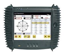
Rugged UMPC for industrial on-site. The UMPC offers protectors, shockproof design, holder for hand/arm.
