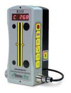
The R310 measures the position of the rotating laser beam. The CCD Sensor has total measurement range of 80mm. The beam forms an entire reference plane. The R310 is wireless and can measure up to a distance of 80m from the Laser.
