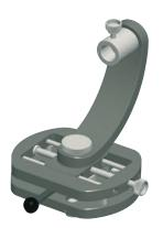
Using the swivel and tilt adapter you can align the laser level, irrespective of the surface below. The Adapter also allows for a parallel movement which is very useful when aligning the laser parallel to a reference object. The Adapter is accommodated with a 5/8" thread, and is also fitted with a three-point magnet arrangement underneath.
