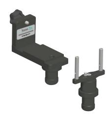
This adapter set is of great practical help for measuring flange parallelism. There is an adapter for the R525 Receiver and an adapter for the T330 Laser. After measuring the first flange, the adapters with their Sensors are exchanged, the tripods are remaining at their position. After re-aligning, the second flange can be measured parallel to the first.
