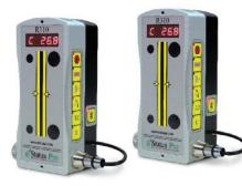
The R310 measures the position of the rotating laser beam. The CCD Sensor has total measurement range of 80mm. The beam forms an entire reference plane. The R310 is wireless and can measure up to a distance of 80m from the Laser.
