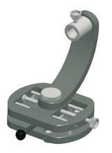
Using the swivel and tilt adapter you can align the laser level, irrespective of the surface below. The Adapter also allows for a parallel movement which is very useful when aligning the laser parallel to a reference object. The Adapter is accomodated with a 5/8" thread, and is also fitted with a three-point magnet arrangement underneath.
