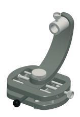
Using the swivel and tilt adapter you can align the laser level, irrespective of the surface below. The Adapter also allows for a parallel movement which is very useful when aligning the laser parallel to a reference object. The Adapter is accommodated with a 5/8" thread, and is also fitted with a three-point magnet arrangement underneath.
