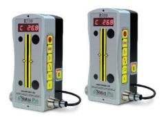
The R310 measures the position of the rotating laser beam. The CCD Sensor has total measurement range of 80mm. The beam forms an entire reference plane. The R310 is wireless and can measure up to a distance of 80m from the Laser.
