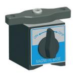
Block magnet (BT 943092) complete with a cross-bridge. This enables the mounting of a R525 Sensor or T250 laser with adapter BG 830780. Available attachment rods: BT 948155, BT 948156, BT 948157
