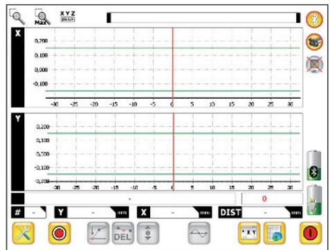
Here you will see information concerning the angle of the detector, the X and Y coordinates. By pressing Zero at the start, then rotating the sensor through 180° and finally halving the value at 180°, you receive the position of the laser beam in respect to the centre of the bore – enabling adjustment accordingly.
