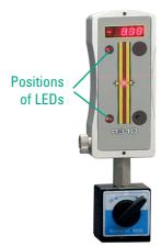
Additionally, the Position LEDs(C) show if the laser beam is above or below Zero. If the laser beam is within +/- 0.1mm of the Zero, both LEDs will blink. This feature is useful when aligning the laser to a reference line over greater distances where the actual measurement value is not visible.
