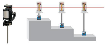
Sometimes when levelling, objects of differing height have to be measured in relation to each other. To enable this, use spacers (FIX 1-0658) placed between the magnet and the M8 Adapter. Typically, you would manufacture the spacers to the exact height difference between the objects, enabling a "Zero" reading when the goal is reached.
