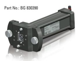
The R525 is a rugged but precise 2D Laser-Position detector. It was developed originally for machine tool alignment applications. Because of the Wireless interface and its versatility it used today in a multitude of applications. Together with the ProLineV2 Software application we measure XY und Z simultaneously. If we use the T330 as a laser source we have a reference which automatically levels itself. These features together are very powerful and save a great deal of time on-site.
