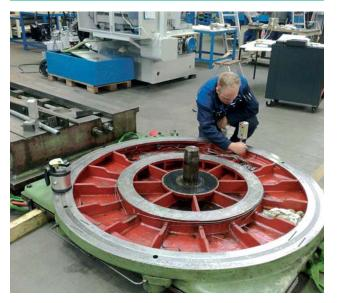
Flange Flatness Measurement is an important variation on the flatness theme and requires special attention. **ProFlange** is a software package which addresses these issues. You do not have to level the flange before measurement or ensure that the reference is parallel.
