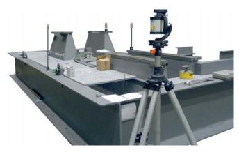
The **T310** creates a flat and level laser reference plane. We use the **R310** with its 80mm detector length to measure against this reference. The Software **ProLevel** lets you place these measurements on a template on site.
