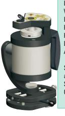
**Technical Data** Laser: Class 2 Weight: 2400 a Body: Aluminium Range: 100 m Rotation: 2 to 10 Hz Dimensions: 125 x 170 x 185 mm with external R310 Ref: Accuracy: <0.005 mRad (mils/in) Self-leveling accuracy: ± 0.02 mRad (mils/in) Step error: typical 0.03 mm Conical error: typical  $\pm$  0.01 mRad (mils/in)
