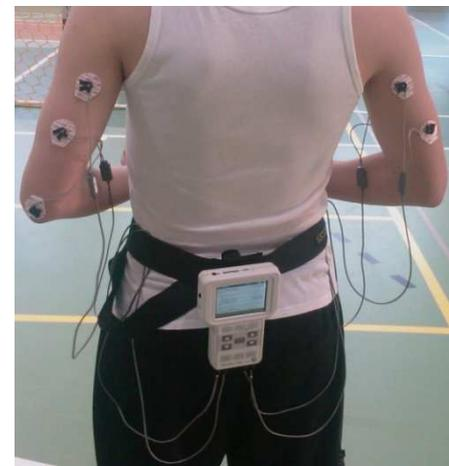
Fig. 4. Arrangement of electrodes during EMG testing – rear view
