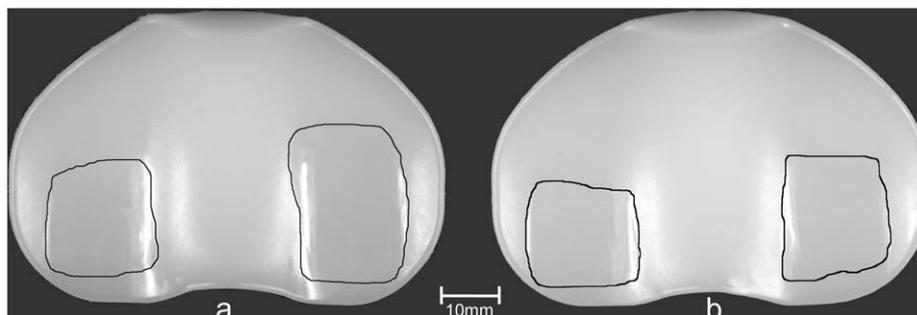
Fig. 5. Wear scars on the superior surface of the tibial inserts are larger when simulating non-linear soft tissue motion restraints (a), compared to the 14243-1:2002(E) conforming linear motion restraints (b).
