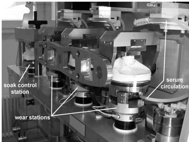
Fig. 4. Experimental setup: AMTI knee simulator with wear and soak control stations as well as serum circulation system.
